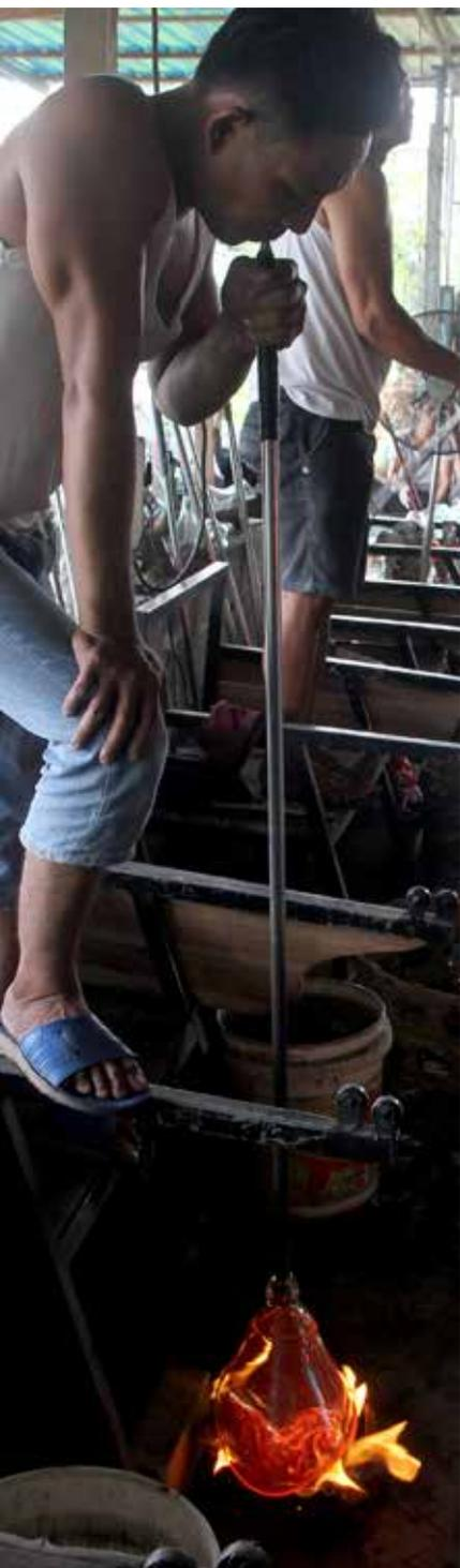
In a village in the hills above Ubud in Bali is a glassblowing workshop. Adding to the tropical heat, the temperature by the furnaces is unbelievable. The artisans work quickly. In one corner two women are preparing broken sheet glass for recycling. Close by four men are rushing to and fro heating the glass until it glows, then deftly blowing it and turning it to create an extraordinary range of shapes.
